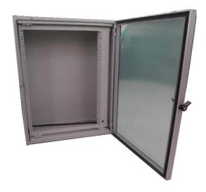
A range of Wall Mounted Cabinets with a swing out frame sealed to IP54. The cabinets are supplied with 19" mounting rails on an internal swing out frame to provide access for cable routing and to internal equipment. The cabinets have a lockable steel framed acrylic glass door for safety and security. The cabinets are available in heights of 380mm, 600mm and 760mm (6U, 11U and 14U).
